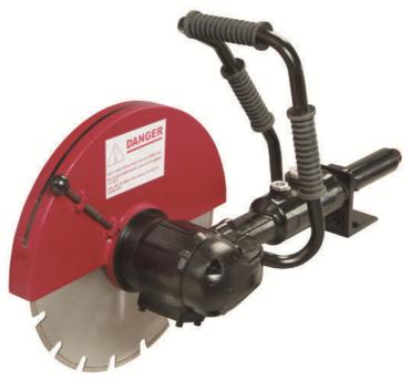
The CP 0044 is a very powerful and durable air tool, driven by a direct drive, 4 hp motor. The direct drive eliminates the need to continuously check the drive belt tension. For use by companies performing indoor cutting tasks in concrete, asphalt, stone, etc. Foundries and other worksites where the use of gasoline powered saws is restricted. General contractor companies.
